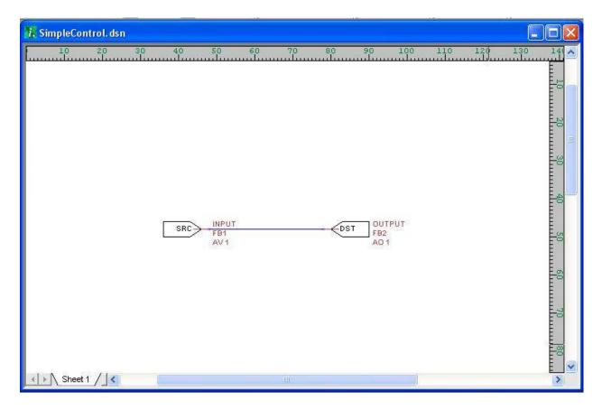
Using the i.CanDrawIt tool, compile the file to create a .plx file. Then from the PL/i tab of the configuration tool, open the .plx file, and click Write to send the program to the ValuPoint. Once that is done, select Run Program from the Program Change list and click Send. The program should now be running, which you can verify by clicking the Read button. The status should appear as follows:
