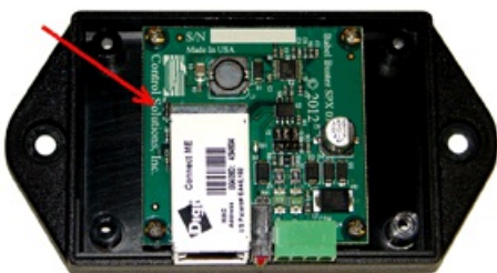
Babel Buster SPX The jumper is found next to the server module at the corner opposite the terminal block. Remove 4 screws from the bottom of the SPX to remove the cover.
